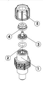
Figure 13 Dischange line with check-valve and ball bearing
