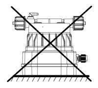
Figure 8 Pump Wrong Assembly Position
