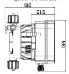
Figure 3 Pump side size
