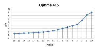
Figure 20 Optima 415 Pump flow rate pressure graphics
