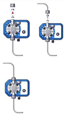
Figure 11 Installing the hose to the pump head
