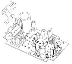
Figure 18 Fuse location on the electronic board Replace the glass fuse shown in the figure, on the electronic board.
