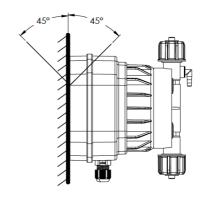
Figure 6 Pump Correct Assembly Position
