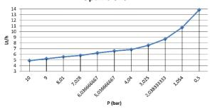
Figure 19 Optima 510 Pump flow rate pressure graphics
