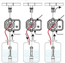
Figure 12 Air vent operation
